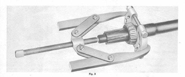
Step 4-Remove the thrust washer.
